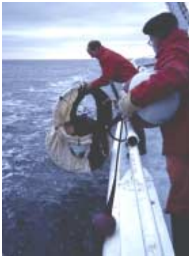
Satellite-tracked surface drifter with float and canvas drogue being deployed off the R/V Wecoma .
