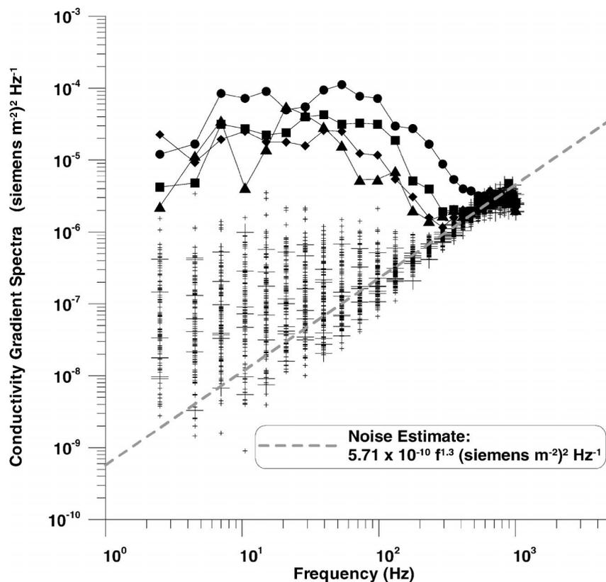
FIG. 5. One-dimensional frequency spectra of  $\partial C/\partial l$  (where  $l$  is in the direction of travel) collected during the spring 1997 CMO cruise. The “+” symbols are from low-signal regions; other symbols are from four sequential high-signal regions. The dotted line is a least squares fit to the spectrum of electronic noise.
