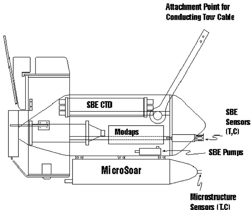
FIG. 1. Schematic diagram of MicroSoar attached to SeaSoar.
