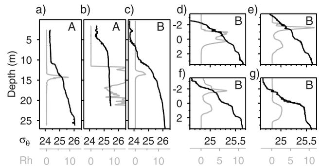
**Figure 4.** Profiles of potential density ( $\sigma_\theta$ ) (black) and rhodamine concentration ( $\mu\text{g/l}$ ) (gray) from (a and b) two downcasts during tow-yo A (west-east) and (c–g) five during tow-yo B (west-east). Figures 4d–4g show an extract from the water column, with depth relative to  $\sigma_\theta = 25.29$ . Profile locations are shown in Figures 3 and 5.
