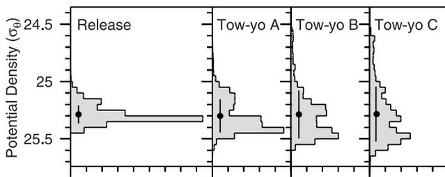
**Figure 2.** Histograms of dye distribution versus density at the time of release (from CTD density during injection), and during tow-yos A, B and C. Distributions are normalized by area. Means and standard deviations are shown by bullets and bars.
