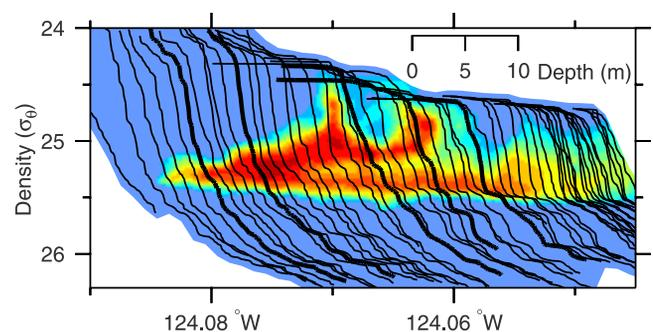
**Figure 6.** Stacked profiles of density against depth (inset axis) during tow-yo B. Individual profiles are offset by the ship longitude (main axis) at the time the CTD crossed  $\sigma_\theta = 25.29$ . Homogeneous layers appear as horizontal steps. The underlying image is of dye concentration, similarly offset by depth and longitude. Bold profiles are those of Figure 4.
