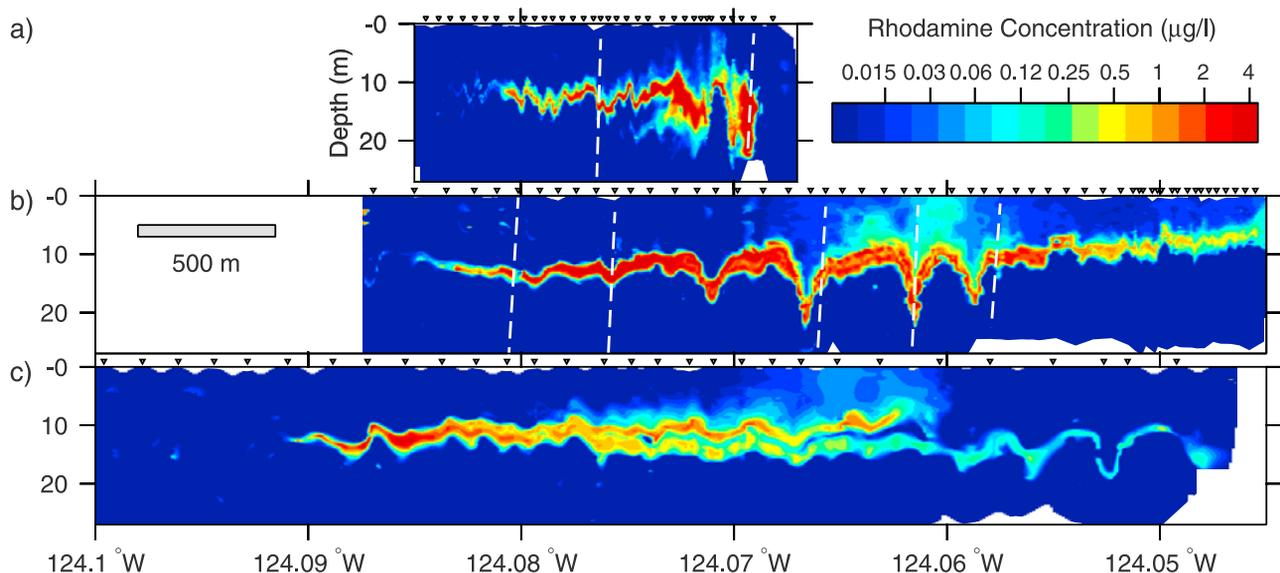
**Figure 3.** Cross-shelf sections of dye concentration from CTD tow-yos. Triangles on the upper axes show the start of each downcast. (a) Tow-yo A, (3.8–5.3 hours post-release), (b) Tow-yo B (12.9–14.7 hours), (c) Tow-yo C, (15.4–17.0 hours). Gridding was performed in  $(x, \sigma_\theta)$  space then transformed to  $(x, z)$  space, a method that favors coherence of the gridded field along isopycnals. Dashed vertical lines show the profiles of Figure 4.
