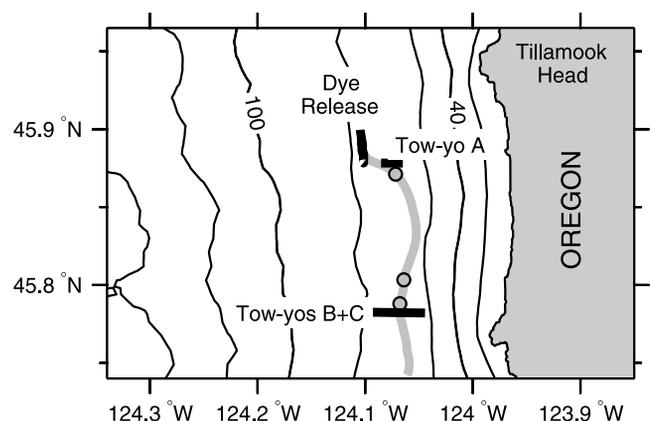
**Figure 1.** Bathymetry (contoured) of the northern Oregon shelf, showing (black) the location of the dye release and tow-yo lines, and (gray) the path of a 15-m drogued drifter released with the dye. Bullets show the drifter position at the mid-time of each tow-yo.
