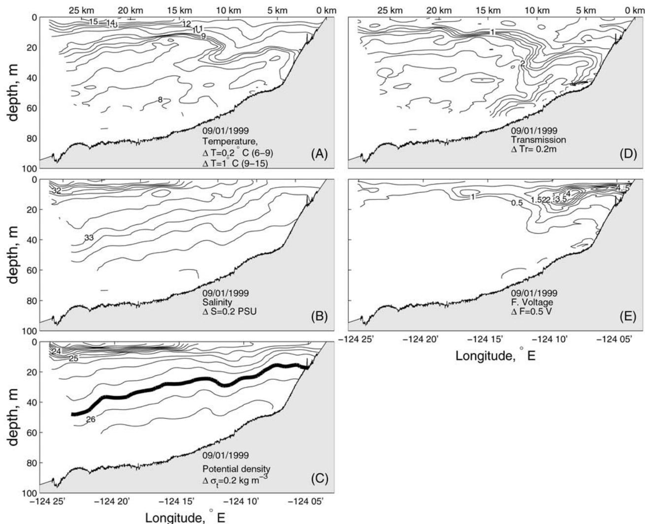
**Figure 5.** Data from the 1 September 1999 cruise taken along  $44.65^{\circ}\text{N}$  (Figure 2, NH line). (A) Temperature. (B) Salinity. (C) Potential density. Heavy line is the  $25.8 \sigma_t$  isopycnal. (D) Transmissivity. (E) Fluorometer voltage.
