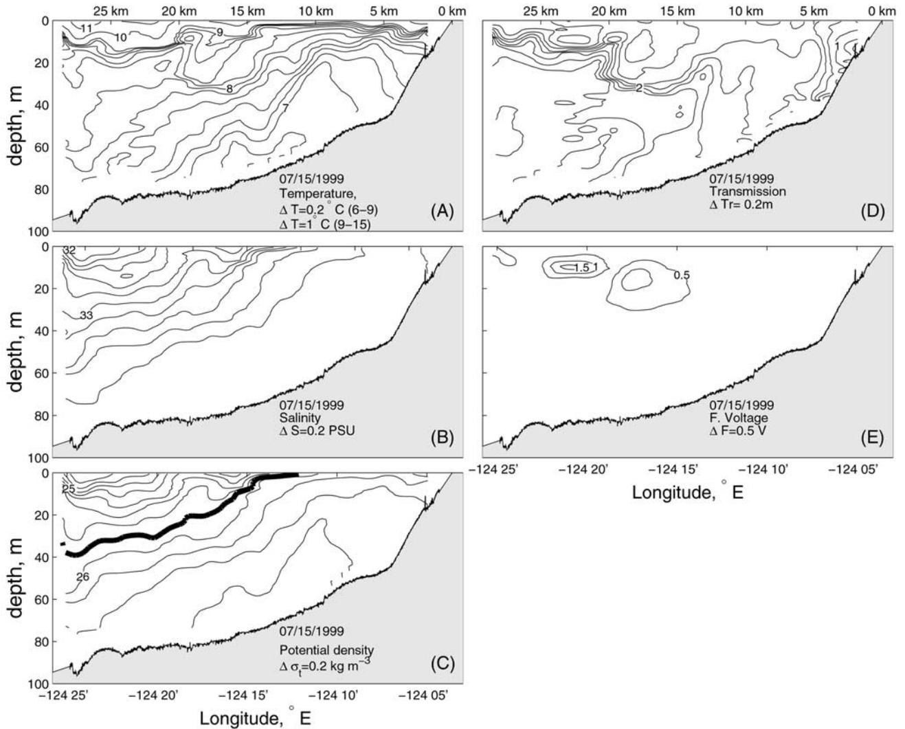
**Figure 4.** Data from the 15 July 1999 cruise taken along  $44.65^{\circ}\text{N}$  (Figure 2, NH line). (A) Temperature. (B) Salinity. (C) Potential density. Heavy line is the  $25.8 \sigma_t$  isopycnal. (D) Transmissivity. (E) Fluorometer voltage.
